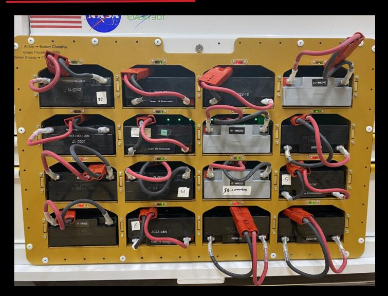
We removed the center 5 drawers of the avionics toolbox with 16 battery charging slots. There are two, <u>10-bank Battery Tender chargers</u> stacked in the back of the toolbox with custom PCBs mounted to the outside of the charger structure to show the charging status of each battery. We generally charge 12 batteries for our robot and the other 4 slots are used to charge batteries for partners, our scouting inverters, and the inverter on the robot cart used to power the drivers station.
